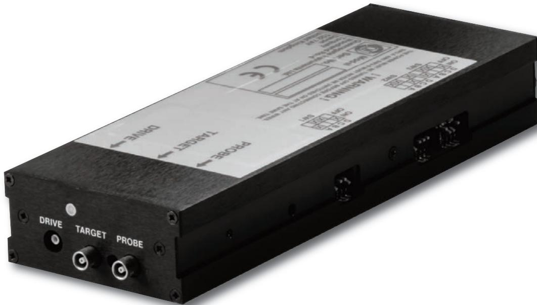
The NPS2101 and the NPS2100-20 are NanoSensor, high voltage amplifier and control electronics combined as a single channel standalone module, powered by an external  $\pm 15V$ , 130V and -30V DC supplies.
