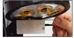
**STEP 3:** Connect the OP400 to the nosepiece. Tighten both grub screws with the hex key.
