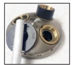
**STEP 2:** Insert the microscope thread adapter using the key provided. Insert parfocal spacer if other objectives are to be used.
