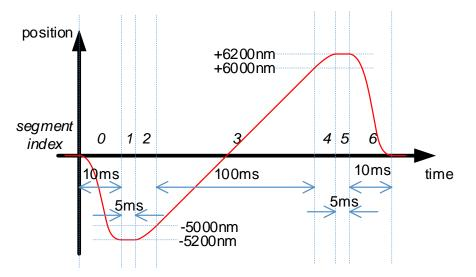
The example above shows a unidirectional linear ramp from -5000nm to +6000nm over a 100ms duration, with start and end considerations around the ramp. This is a typical operation for many applications, for example focussing a microscope. The waveform carries out the following operations:-
