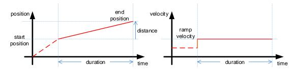
This provides a simple ramp. The user has the choice of whether to ramp over a fixed time or a fixed distance.
