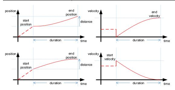
A common technique for minimising resonance during acceleration and deceleration is for the trajectory to follow a portion of a sine wave.
