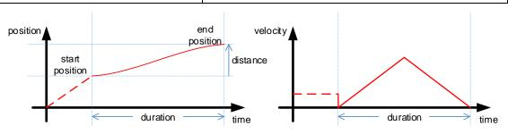
This uses constant symmetrical acceleration and deceleration to round off the edges of a step, which can reduce system resonances. This is an extremely simple profile, but can give reasonable results where more complex trajectory profiles are not required.
