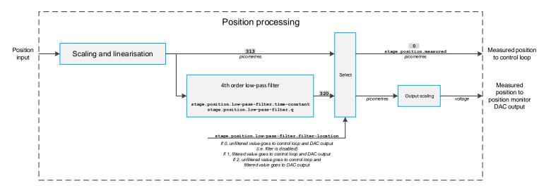
Note that the output scaling from a position in picometres to a voltage on the position monitor output will vary depending on the stage. This scaling is specified in the stage datasheet.
