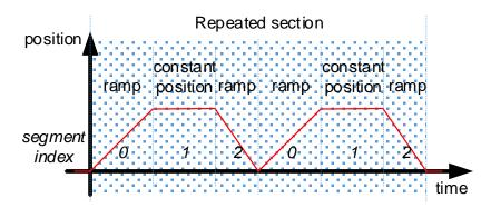
In the example above, the waveform has 3 segments. The start of the repeat section is segment 0 (the first segment) and the end of the repeat section is segment 2 (the last segment), with a repeat count of 2.
