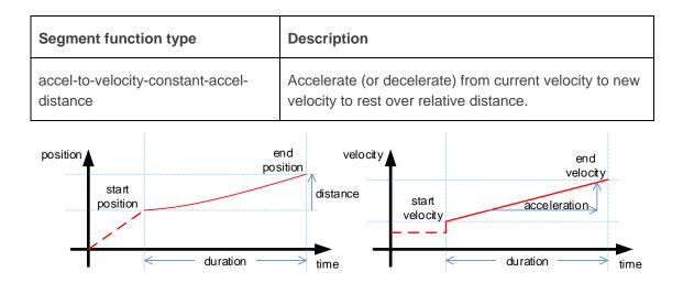
A common acceleration profile for accelerating and decelerating is to apply a constant acceleration/deceleration until the desired change in velocity is achieved. The constant acceleration results in a triangular velocity profile. Acceleration may be specified directly, or the required acceleration may be calculated from the acceleration duration or distance travelled, as required for the user's waveform.
