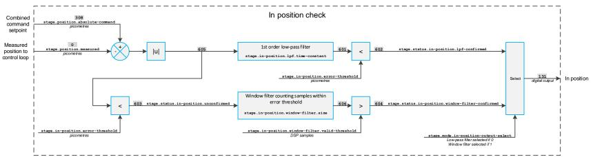
The in position ("ready") check only runs when the control loop for the channel is in closed-loop mode (see 5.11.3, stage.mode.closed-loop). In open-loop mode, the command does not relate to an actual position, so the in position status/output is always false or logic-low in open-loop mode.
